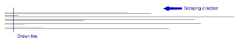
Figure 4 Fabricating debris defects cause fewer scratches near the beginning of the scraper's path. More scratches will be observed near the end.
