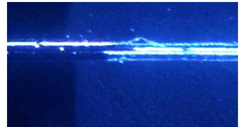
Figure 6 Count all scratches which intersect with the drawn line.
